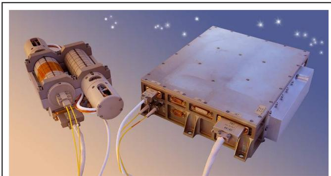
Figure 4. The Absolute Scalar Magnetometer (ASM) : left, two sensors mounted on the bracket. Right, one DPU. Credits : CEA-LETI
