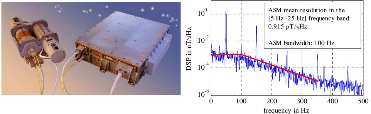
Fig. 2. (a) ASM sensor assembly and ASM DPU; (b) ASM scalar bandwidth and resolution
