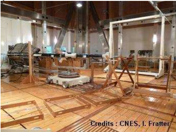
Figure 7 Differential measurements layout during satellite magnetic tests in IABG's MFSA facility
