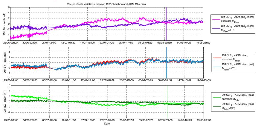
Components peak to peak variations:  $\pm$  2 nT (North), smaller for the other directions, 16° C < T<sub>sensor</sub> < 28 °C; evolution observed mainly during the first weeks after the installation
