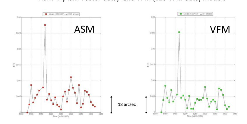
Apparent angular fluctuations between ASM or VFM frames and the STR frame for Alpha (co-estimated with models ASM-V and VFM, respectively)
