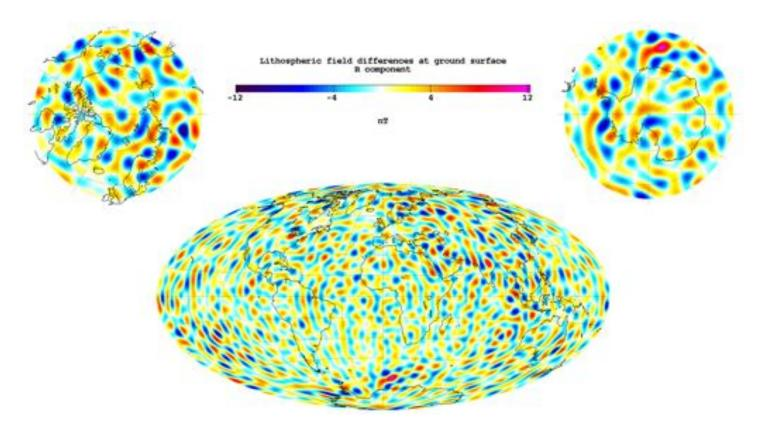
$\Delta$ Br difference at Earth's surface (n=15-45) between ASM-V (ASM vector data) and VFM (L1b VFM data) models
